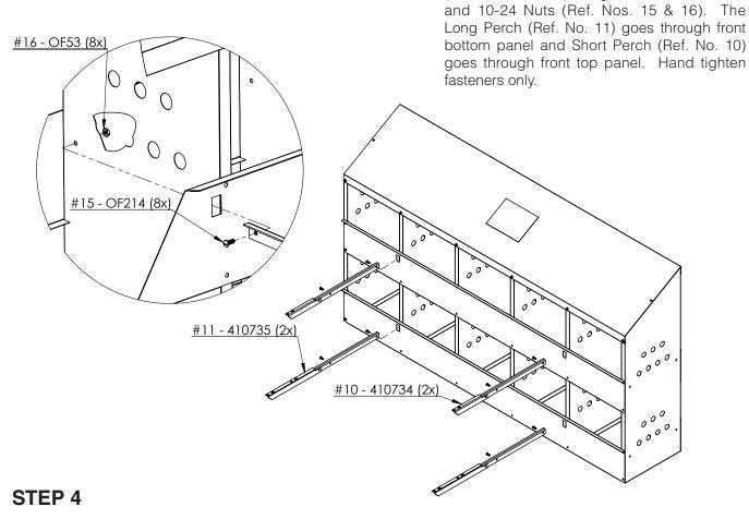
Attach Long and Short Perch Assemblies (Ref. Nos. 10 & 11) using 10-24 Machine Bolts
