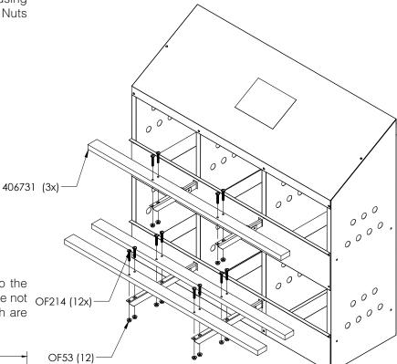
NOTE: The distance of the mount hole to the edge of the Wood Perches (Ref. No. 9) are not the same on both ends. The holes which are 12" from the edge go on the right.
