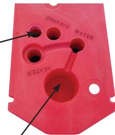
Cavity for warm climate installations only. Some warm geographic areas do not use a riser and may only have a buried supply line protruding through a concrete pad. The cavity can be used to make the connection from the supply line to our valve.
