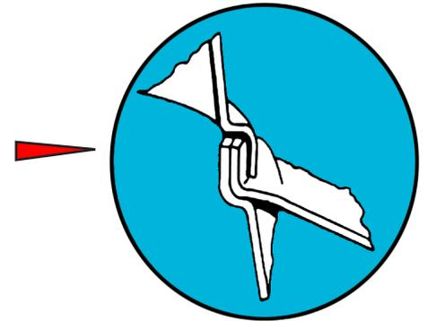
Body has a fall away taper to facilitate feed flow.
