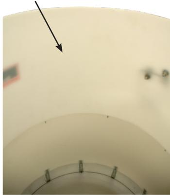
Rain shield extends beyond the trough 6 inches (15.2 cm). Height of the rain shield above trough is about 11 inches (28 cm).
